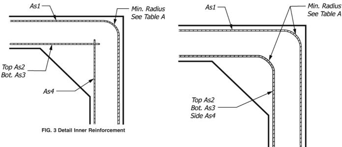
Note 3—(Advisory)—The reinforcing areas shown in Table 1 are based on the design earth covering and live load conditions described within this standard. Depending on the means and methods used, handling and installation loads by either the manufacturer or contractor can induce stresses not considered within the development of the tables. These loads could require additional steel reinforcement beyond the minimums shown within the standard. These handling and installation loads should be
